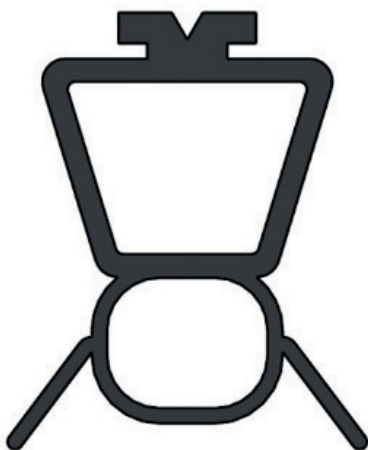
Old type of sealing (material EPDM) BAAN code: T09-020-20-0008
